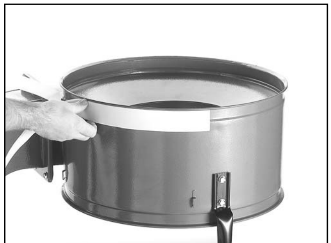
Figure 14. Installing wide foam strip.
